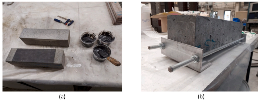
Fig. 1. (a) Gluing of the CFRP laminates on a concrete specimen and (b) concrete specimen inside a metal frame for restraining of the crack width.
