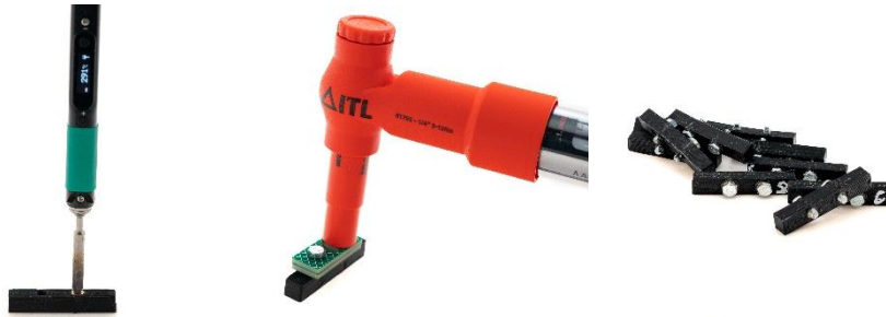
Figure 3-3: Heat threaded insert torque testing
