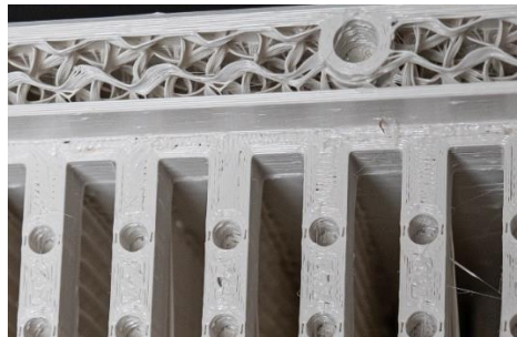
Figure 3-13: Enclosure close up, wall count, and infill pattern are visible
