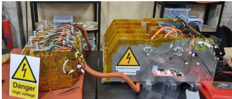
Figure 1-7: UGent Racing 2022 segments and accumulator container
