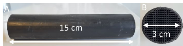
Fig 1. Side (A) and top view (B) image of the used activated carbon monolith, wrapped in heat shrink tubing
