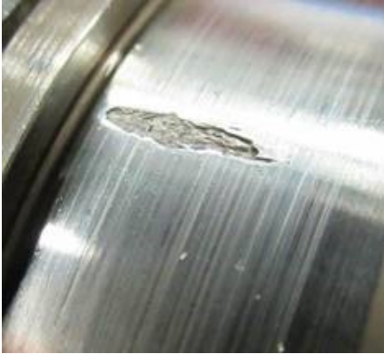
Figure 1. Picture of the damaged inner ring of the rolling element bearing.
