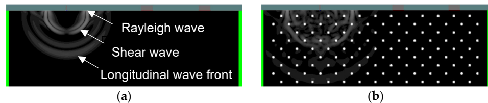
Figure 4. Displacement field close to the surface of (a) mortar without voids and (b) mortar with 3% voids a few \mu s after excitation.
