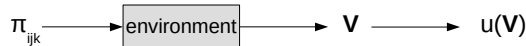
Fig. 5 The execution phase for the Team Reward Team Utility setting. This figure depicts the SER optimality criterion, where the expected values (i.e., the average over many executions of the policies) will be input to u . Under ESR the input to u would be \boldsymbol{\rho} , i.e., the returns for an individual roll-out.
