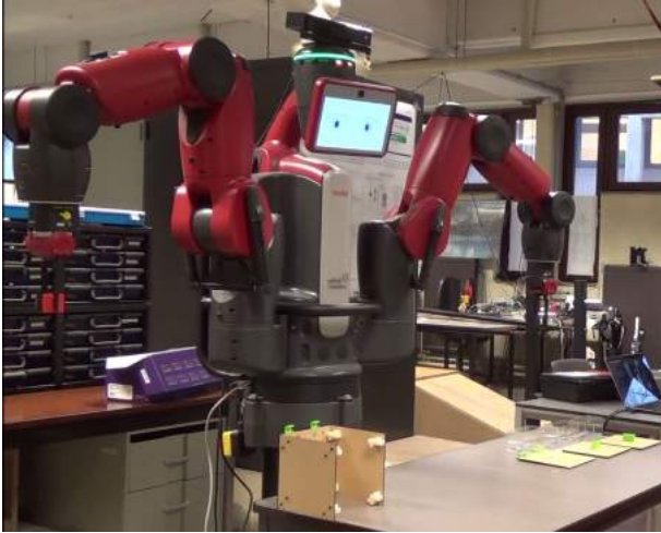
Fig. 1. The collaborative Baxter robot. A Kinect v2 camera is placed on top of the robot for gesture and face recognition. The camera is placed on the robot's head to avoid occlusions by the arms and the parts.
