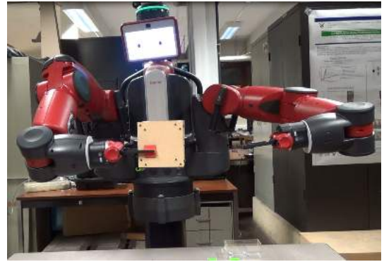
Fig. 4. Baxter checking the number of screws via the wrist camera during the assembly task.
