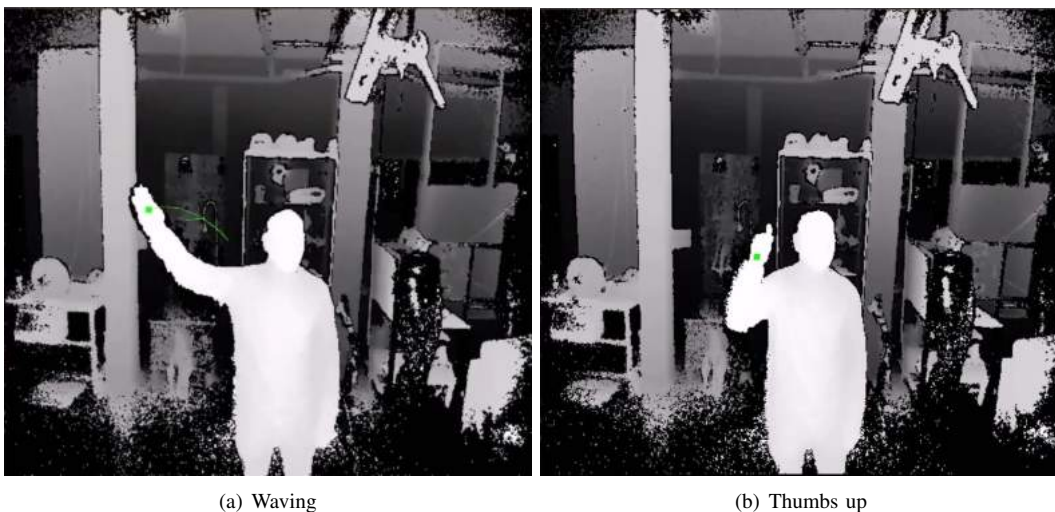
Fig. 2. Depth images during the gesture recognition with the Kinect v2 camera using the NiTE 2.2 interface. Two gestures are shown here: the waving and the thumbs up gestures.
