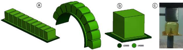
Figure 9 In future work multiple cells will be combined to form a bending soft pneumatic actuator as shown in (a). A soft pneumatic cell in (b), and under test while the resulting force is measured (c).
