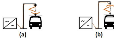
Fig. 1. The two investigated pantograph concepts in this study (a) inverted pantograph also referred to as top-down or infrastructure mounted; (b) roof mounted pantograph also referred to as bottom-up
