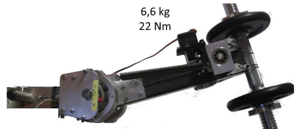
Fig. 6. The final MACCEPA-based SPEA with cylindrical cam mechanism. On the left the motor and cylindrical cam mechanism and self-closing guides. On the right the pretensioning mechanism for variable stiffness.
