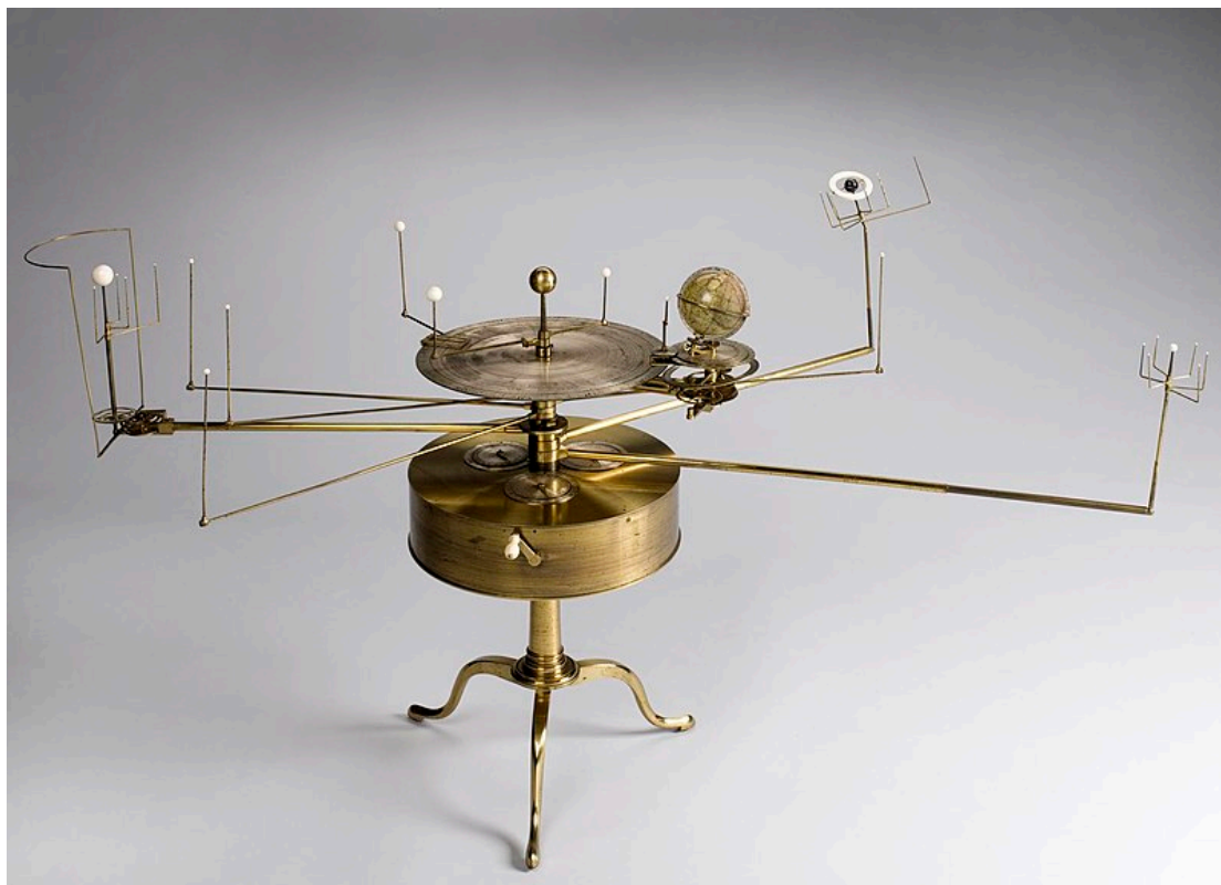
Figure 3: a clockwork mechanism simulating the movements of the planets and their moons. Photo source: Wiki Commons
