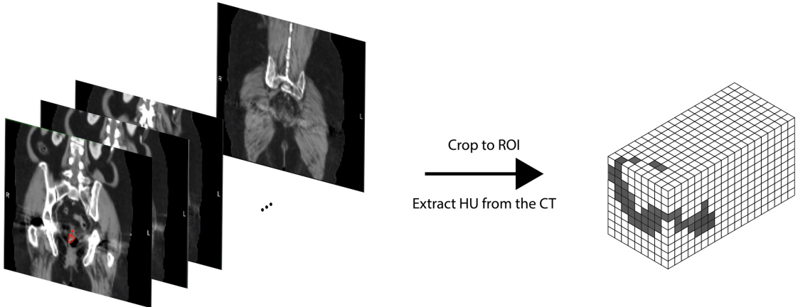
Figure 7.1: Store the ROI from the CT scan as gray-values in a 3D matrix.
