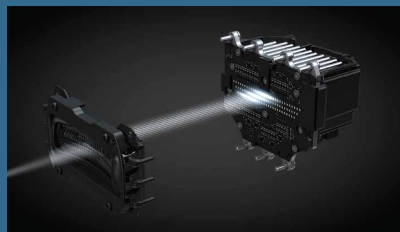
Figure 8: HELLA 84 matrix LED Vehicle Headlight [2].
