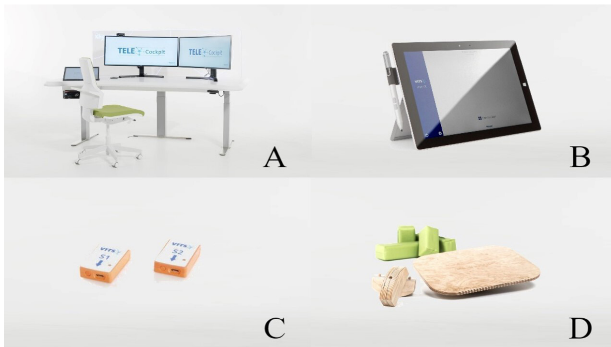
Figure 2 (A) TeleCockpit workstation, (B) VRRS Home Tablet, (C) VRRS Khymu and (D) VRRS Balance. VRRS, Virtual Reality Rehabilitation System.
