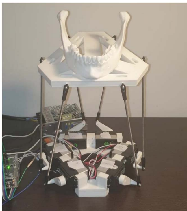
Figure 1. Dynamic six degrees-of-freedom phantom of the mandible.
