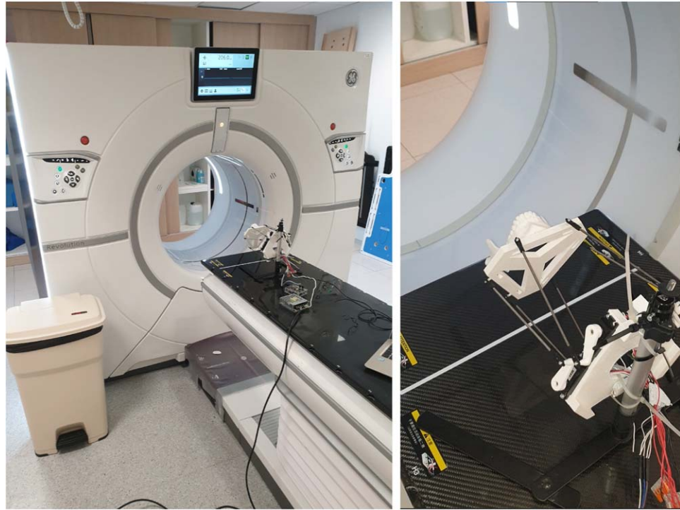
Figure 2. The clinical 256-slice Revolution CT (GE Healthcare, Waukesha, Wisconsin, USA) (left) which was used to obtain continuous scans without table movement while the phantom (right) was in motion.
