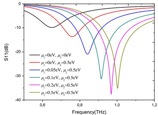
Figure 3. Reflection coefficients of the dipole antenna versus frequency for different chemical potentials of graphene.
