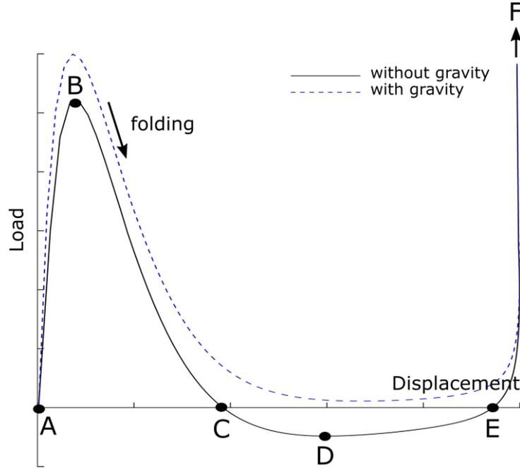
Figure 2: Schematic load-displacement curve of a bistable scissor structure with and without considering gravity.
