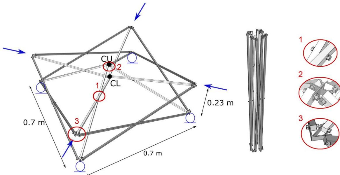
Figure 1: A square bistable scissor module in the deployed configuration with the applied loads and boundary conditions (left) and in the folded configuration (middle) and a detail of the different connections (right).
