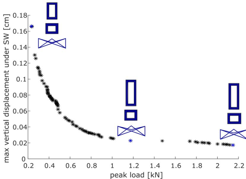
Figure 5: Pareto front and the design variables (from top to bottom: cross section of the outer beams, cross section of the inner beams and structural geometry) for three solutions.
