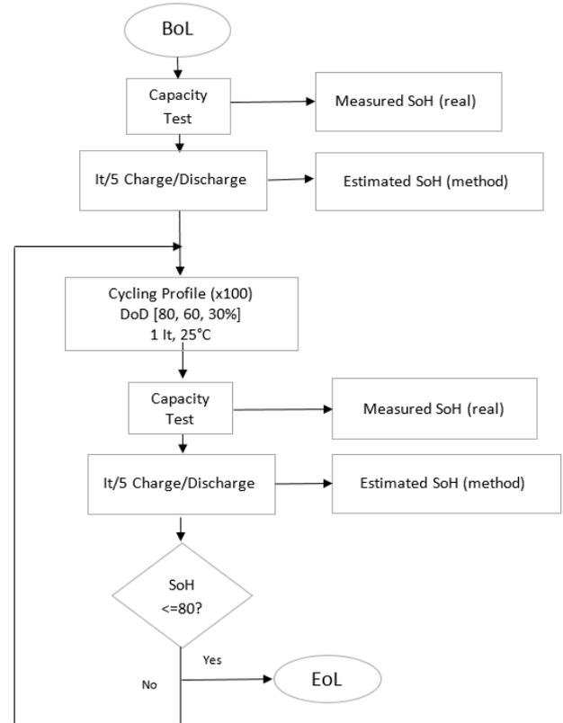
Figure 1: Flow chart, testing procedure.
