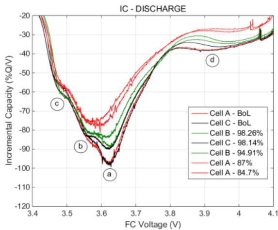
Figure 2: Evolution of IC curves obtained from the tested cells in terms of aging [17].
