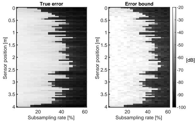
Fig. 3. True error and estimated error bounds over the different scanning positions and for increasing sampling rates.
