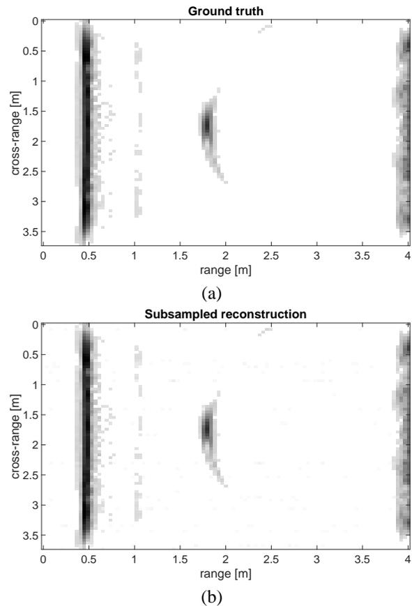
Fig. 5. (a) Reconstructed range profiles with 100% of the samples. (b) Reconstructed range profiles with a mean subsampling rate of 18%, distributed over the different scanning positions as depicted in Fig. 4.
