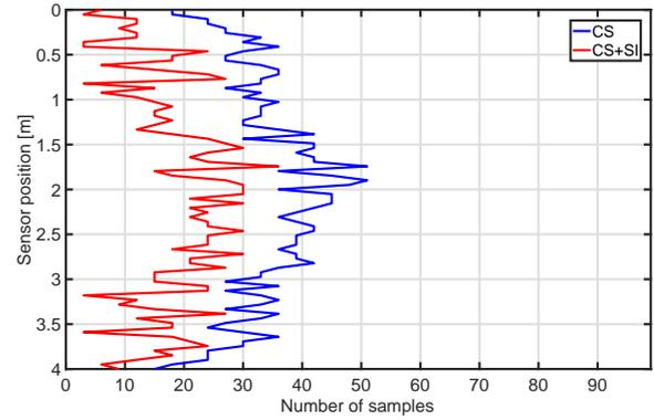
Fig. 4. Number of Samples, over the different scanning positions, required to satisfy a maximum reconstruction error of  $-35\text{dB}$  by applying CS with (red curve) and without (blue curve) weighted SI.
