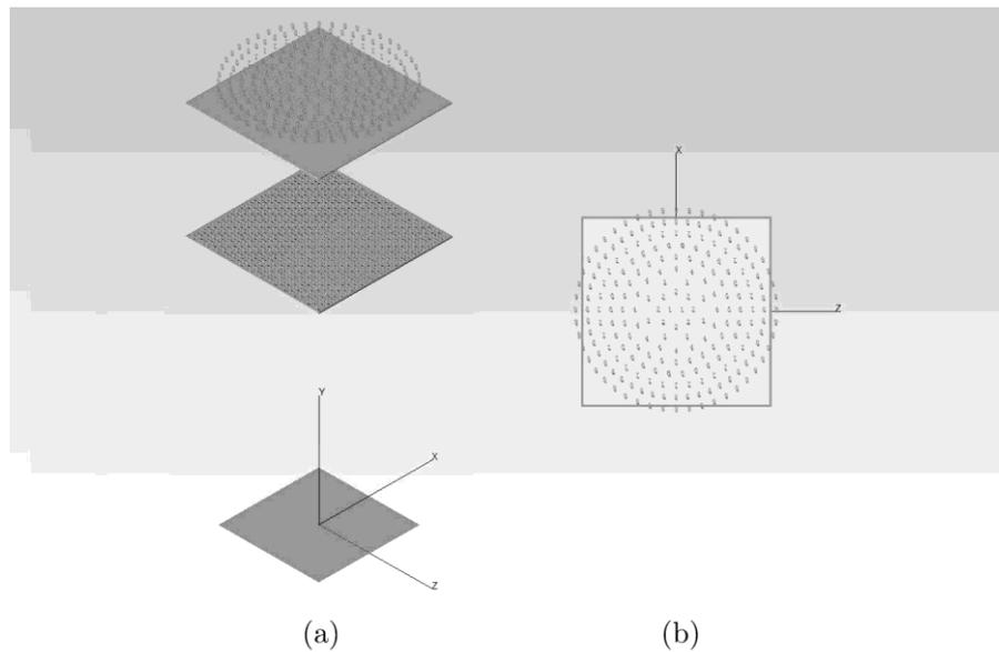
**Figure 2 – (a) 3D view of the optical design for the new surgical luminaire. Above, the 214 LEDs can be found, followed by a non-perforated polycarbonate plate, followed by a perforated plate as described earlier. Below a measurement plane can be seen. (b) top view.**
