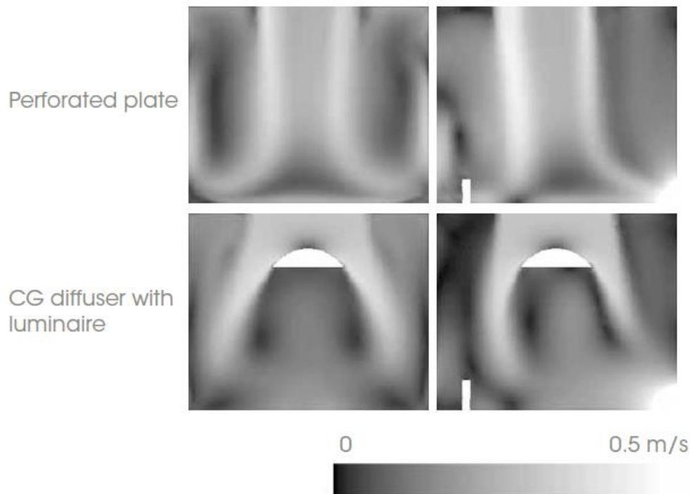
**Figure 3 – Comparing the airflow of the newly designed system using perforated plates with a conventional laminar flow system with CG diffuser and a luminaire, it can clearly be seen that the airflow displays a more stable behaviour in the new system. Figure courtesy of Romy Van Gaever.**
