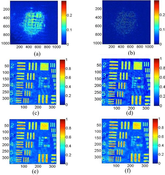
Fig. 3 (a) Amplitude of wavefront  $g$ ; (b) amplitude of  $g_M$  (15% subsampling rate); (c) reconstruction by BP from  $g$ ; (d) reconstruction by interpolated BP from  $g_M$ ; (e) CS with Haar wavelet; (f) CS with CDF 9/7 wavelet.
