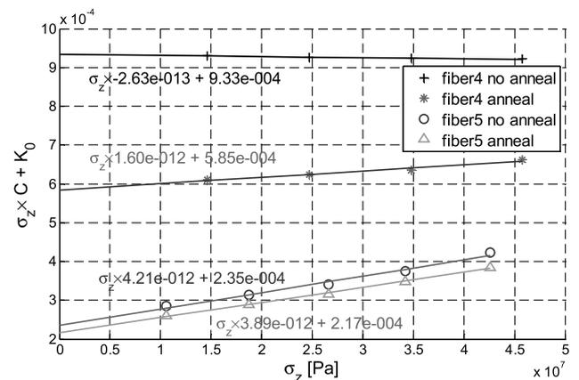
**Fig. 3.**  $\sigma_z \times C + K_0$  as a function of the axial stress measured on samples of Fibers 4 and 5. The values of  $C$  and the extrapolated values of the residual stress are indicated in the graph along the respective linear fits.
