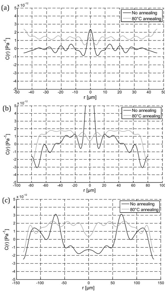
**Fig. 2.** Comparison of the radial distribution of the photoelastic coefficient  $C(r)$  of the POFs under test without annealing and with 8 h annealing at 80°C in (a) Fiber 1, (b) Fiber 2, and (c) Fiber 3.
