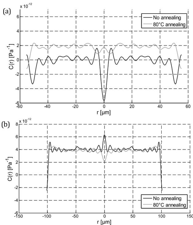
**Fig. 4.** Comparison of the radial distribution of the photoelastic coefficient  $C(r)$  of (a) Fiber 4 and (b) Fiber 5 before and after 8 h annealing at 80°C.
