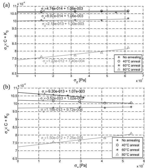
**Fig. 1.**  $\sigma_z \times C + K_0$  as a function of the axial stress measured on a sample of (a) Fiber 1 and (b) Fiber 2. The regression coefficient is the mean photoelastic constant  $C$ . The values of  $C$  and the extrapolated values of the residual stress are indicated in the graph along the respective linear fits.
