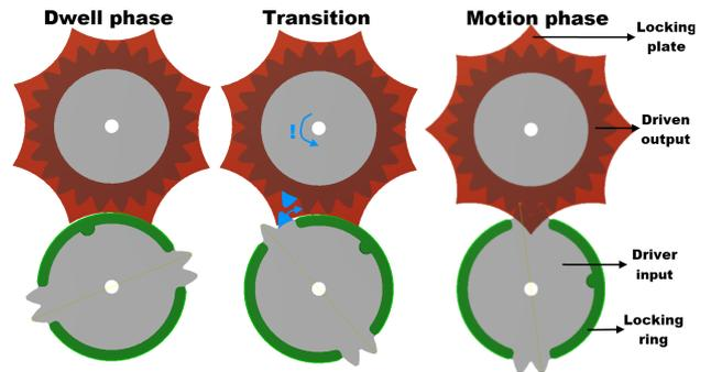
Fig. 3. Schemes of a pair of mutilated gears in the dwell, transition and motion phase. The potential blocking under load is illustrated by the two light blue teeth in the transition phase.
