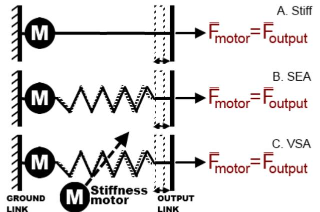
Fig. 1. Actuator schemes to illustrate that  $F_{\text{motor}} \cong F_{\text{output}}$  for a stiff actuator, a SEA and a VSA.
