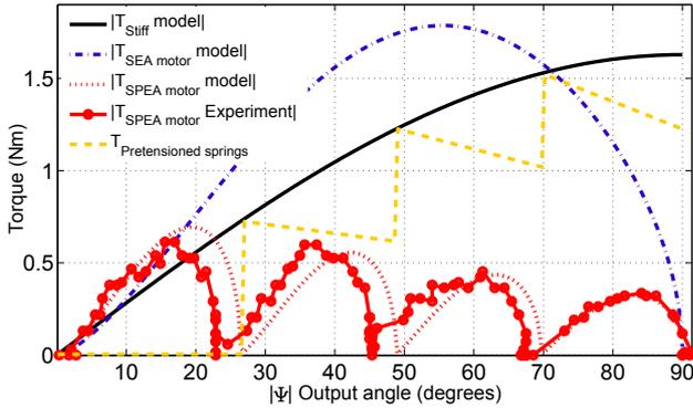
Fig. 7. The motor torque of the SPEA with 4 springs is clearly lower than the motor torque of the equivalent stiff and the SEA set-up. The measurements clearly match the modeled trend of reduced motor torque compared to the stiff and SEA set-ups.
