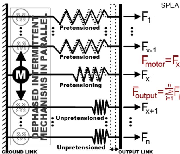
Fig. 2. Principle scheme of a SPEA with dephased intermittent mechanisms in parallel. In comparison to the actuators in Fig. 1,  $F_{motor}$  is only a fraction of  $F_{output}$  for a SPEA.
