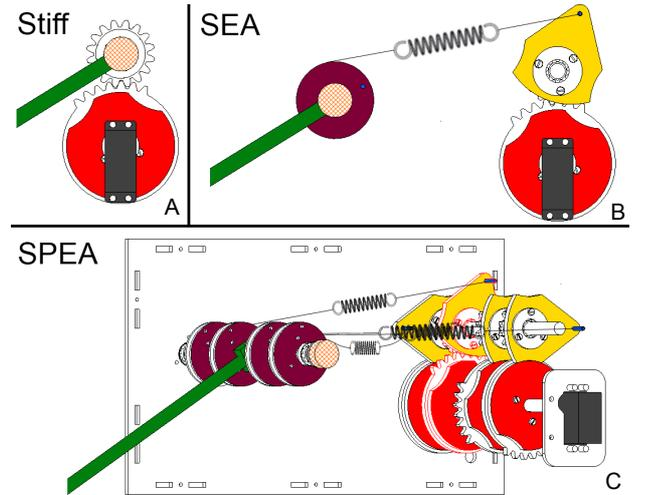
Fig. 6. The SPEA set-up with 4 springs in C, equivalent SEA in B and stiff set-up in A.
