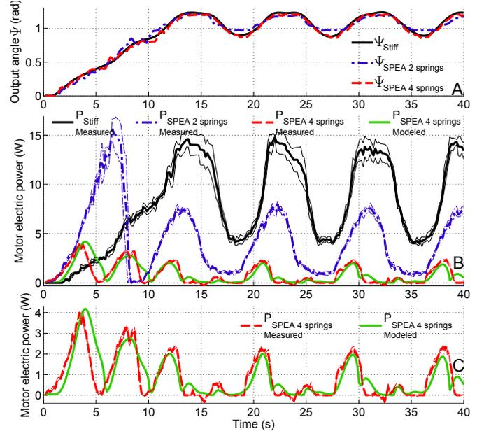
Fig. 8. A: The measured output angle for the three set-ups of the motor power experiment is comparable. B: The decrease in measured electric motor power as a function of parallel springs in the SPEA is clearly illustrated. C: The modeled electric motor power in a SPEA with four springs approximately matches the measurements.
