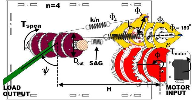
Fig. 4. All relevant SPEA parameters indicated on a scheme of the PoC.
