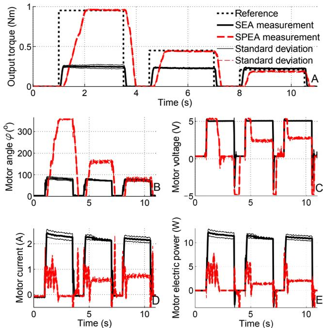
Fig. 9. Open loop output torque tracking experiments of the SPEA PoC and SEA with the output angle  $\psi$  constant at  $0^\circ$ . The measured output torque is given in A. The measured motor data is given in B,C,D and E.
