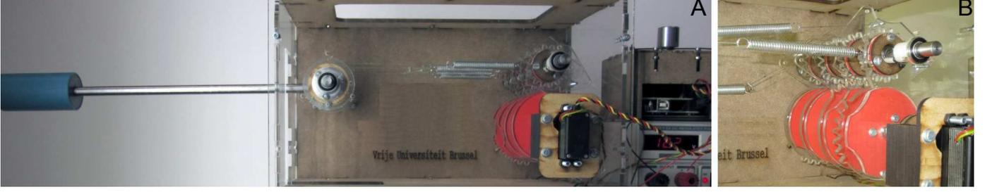
Fig. 5. Overview picture of the SPEA PoC (left) and a close-up of the mutilated gears (right).
